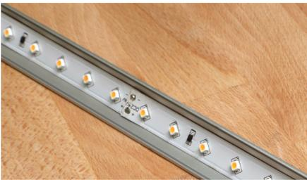
3. Insert the tape light into the channel by peeling off the cover on the adhesive backing and pressing the tape in a straight line from one end of the channel to the other to ensure flat, even adhesion.
